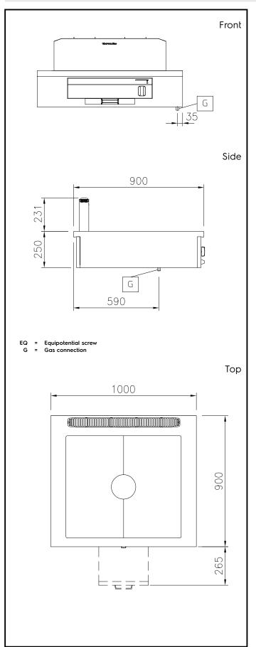
Gas Gas Power: 589580 (MCLIAAJOPO) 12.5 kW Gas Type Option: Gas Inlet: 1/2" **Key Information:** Configuration: One-Side Operated;Top Solid top usable surface (width): 790 mm Solid top usable surface (depth): 700 mm External dimensions, Width: 1000 mm External dimensions, Depth: 900 mm External dimensions, Height: 250 mm Net weight: 120 kg
